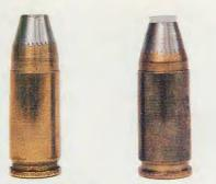
"Cyclone" tubular steel rounds, designed to defeat polyaramid fabric body armor: At left is prototype bullet loaded in Winchester brass for U.S. Army at Aberdeen Proving Ground, Maryland. At right is similar bullet loaded in GEA brass with a highdensity polyethylene feeder-tip to facilitate functioning in automatic weapons.
